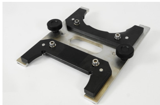
Overlay Test specimen jig
