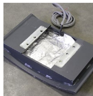
Heating system incorporated in mould base support
