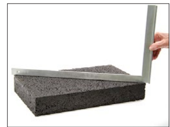
Optimally compacted sample that features planary regularity and homogeneity (PRO)
