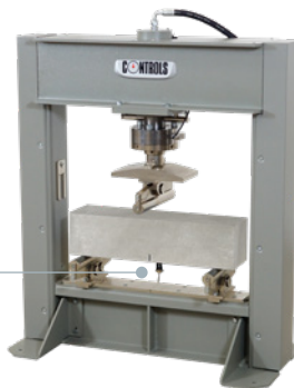
Deflection test on Steel Fiber Reinforced Concrete beams to EN 14651 [CMOD Method] and to UNI 11039 (CTOD method)
