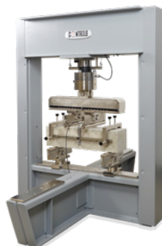
Deflection test on Steel Fiber Reinforced Concrete beams to EN 14651 [CMOD Method] and to UNI 11039 (CTOD method)
