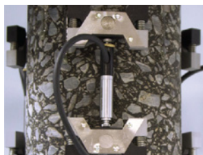
Detail of AASHTO T378 dynamic modulus configuration
