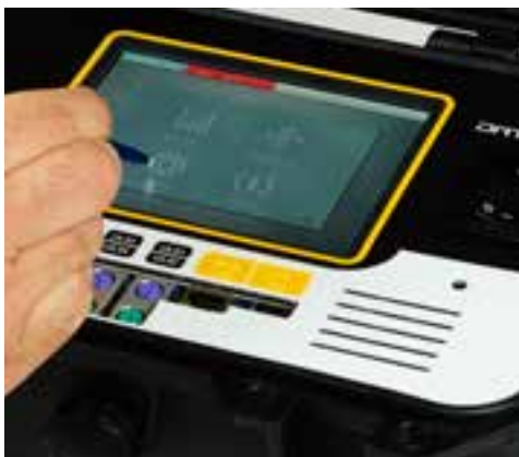
Data acquisition unit DATALOG 8 model 82-P9008/F - Detail of the 6" touchscreen color graphic display
