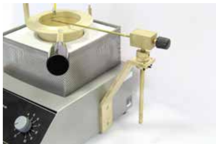
81-B0130/C Brass cup mounted on the electric heater
