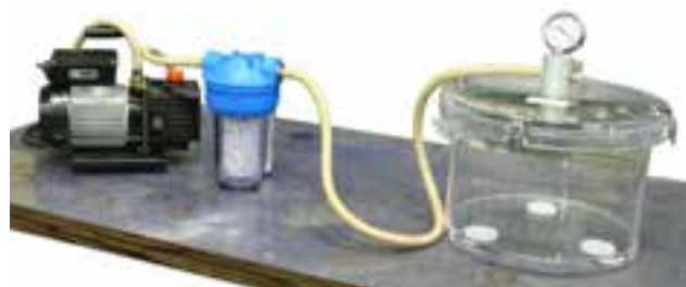
Typical application of 86-D2005 during the determination of the maximum density of bituminous mixtures using the large size pycnometer 75-D1122
