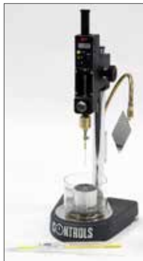
81-B0100/D with Needle, Mirror, Glass transfer dish, Sample cup and thermometer
