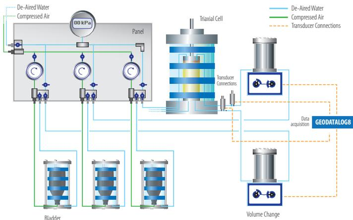
**Permeability tests in triaxial cell with contaminated water**
