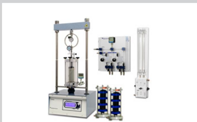
■ **Triaxial System with analog measurements** is the ideal basic solution to perform standard triaxial tests, such as effective and total stress, for laboratories that don't require digital measurement. All the data acquisition and test management are made in manual mode.
