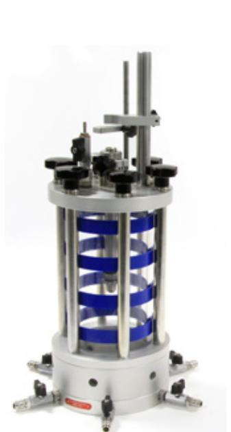
Banded triaxial cell 28-WF4070 fitted with upgrading kit 28-WF4070/ADV for using bender elements and local strain transducers
