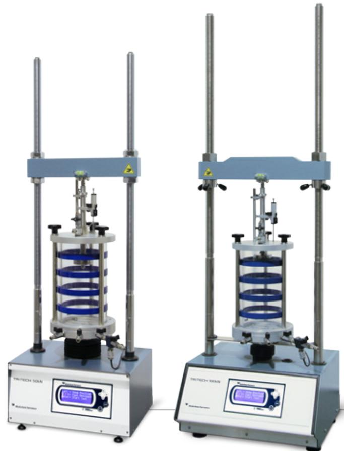
TRITECH 50 and TRITECH 100 fitted with banded triaxial cell submersible load cell and pore pressure transducer
