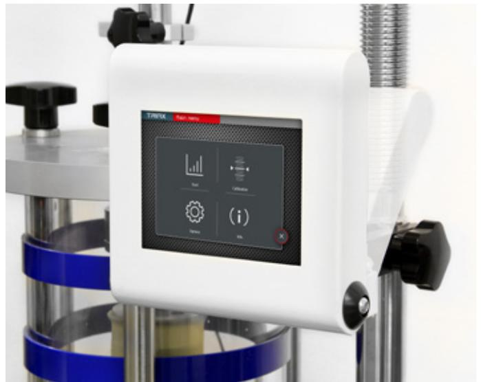
The touchscreen controller is mounted on an ergonomic, multi-jointed support that allows its position to be adjusted in four different ways: changing the height of the support; rotating the support (a); swiveling the touchscreen (b); tilting the touchscreen (c)
