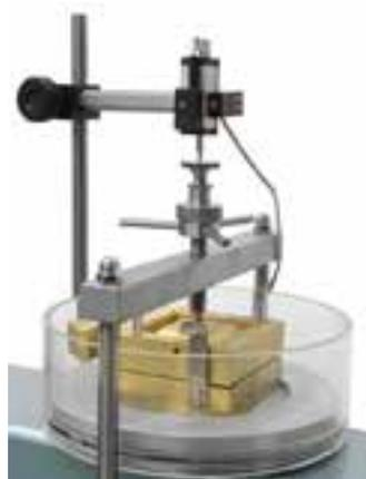
Detail of shear box case fitted in electronic mode
