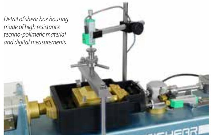
Detail of shear box housing made of high resistance techno-polimeric material and digital measurements
