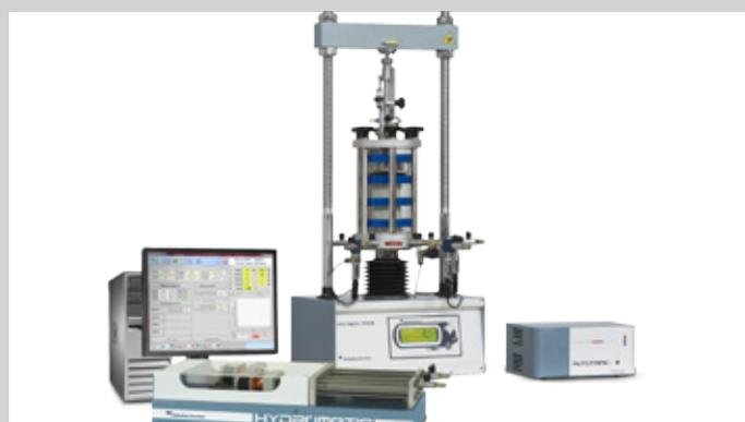
■ **Triaxial System with automatic external data acquisition** is the expandable compact solution for standard triaxial testing (effective and total stress) and for many other soil tests. It can be equipped with standard air/water interface pressure system or with automatic pressure/volume controllers. Data acquisition can be shared with other soil testing equipment (e.g. consolidation and shear) acquisition and/or PC.
