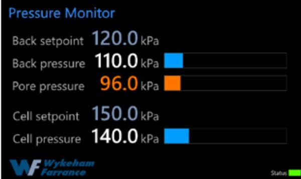
Cell, back and pore pressure monitoring via high resolution 7" color touchscreen display
