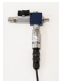
Pressure transducer with de-airing block
