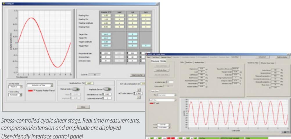
*Stress-controlled cyclic shear stage. Real time measurements, compression/extension and amplitude are displayed
