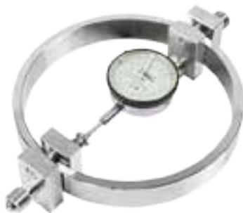
27-WF1002/ST load ring with adapter
