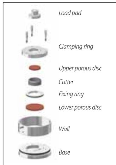
*Exploded view of consolidation cell 26-WF0320*
