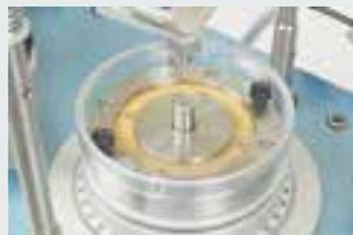
*Detail of 40 cm<sup>2</sup> stainless steel ring shear box fitted with easily removable sintered porous stones with specialized pattern design.*
