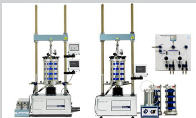
■ **Triaxial System with automatic built-in data acquisition** is the simplest compact solution for standard triaxial testing (effective and total stress). It can be equipped with standard air/water interface pressure system or with automatic pressure/volume controllers. No requirement for external data acquisition and/or PC.
