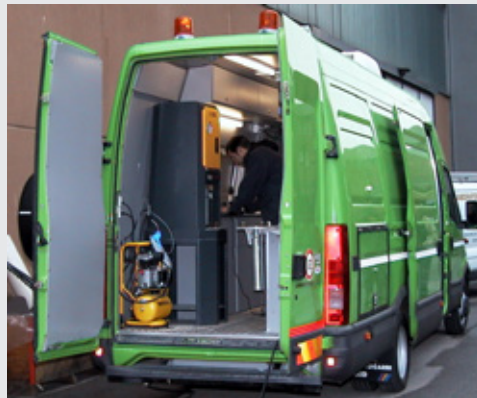
Example of AUTOLAB for road testing. On the left our Gyrotory compactor.
