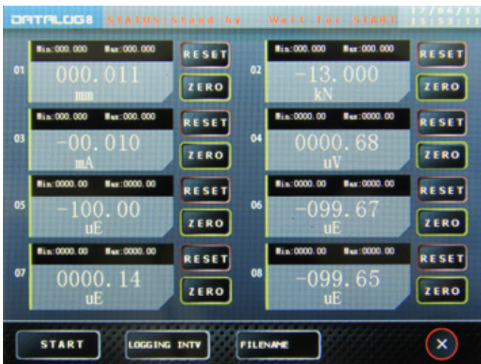
Data acquisition unit DATALOG 8 model 82-P9008 and 82-P9008/F - Live readings of the 8 channels
