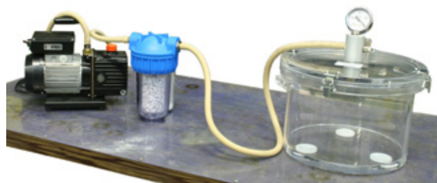
Typical application of 86-D2005 during the determination of the maximum density of bituminous mixtures using the large size pyknometer 75-D1122
