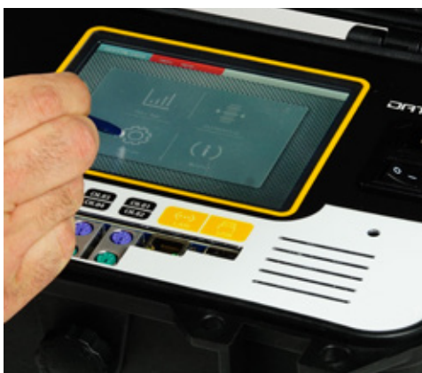
Data acquisition unit DATALOG 8 model 82-P9008/F - Detail of the 6" touchscreen color graphic display
