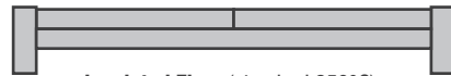
Insulated Floor (standard 250°C) Oven floor raised 100mm with reinforced insulated base
