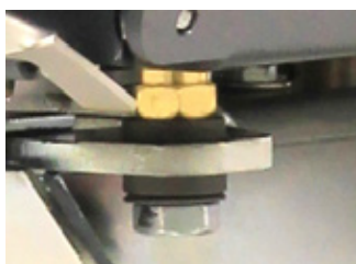
Detail of the 3-point mechanical device to precisely adjust the gap between bowl and beater conforming to Standards
