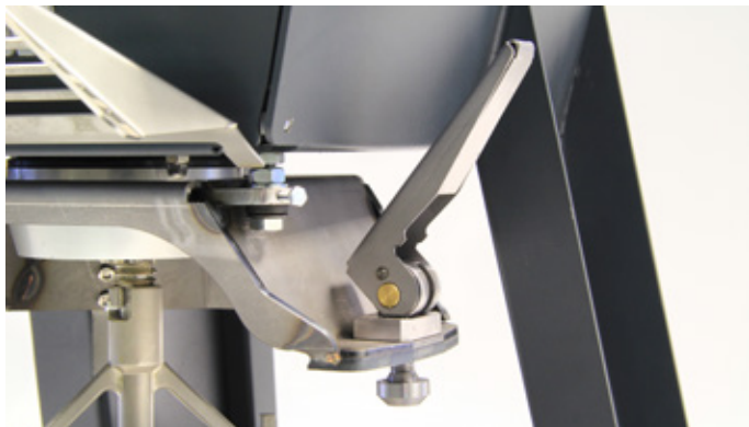
Device for fast and easy lock/unlock the bowl
