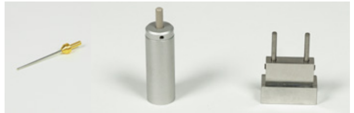
2mm needle to ASTM C807 (63-L2700/F21) on the left; consistency probe and additional weight to ASTM C807 (63-L2700/F15) on the right
