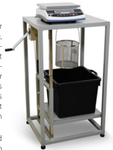
11-D0612/C with 11-D0612/1 Density basket and 11-D0630/30 electronic balance
